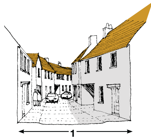
minimum 5.8 wide shared surface special surface to encourage slower speeds
