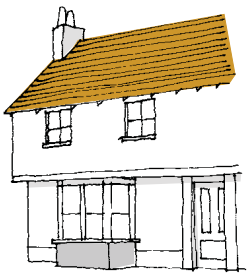
Overhanging jetty allows more flexibility of fenestration
